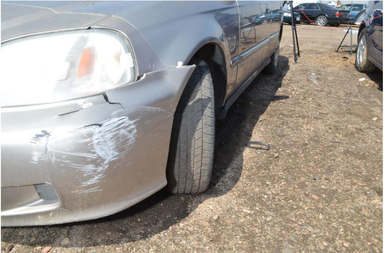
This shows the position of the front wheel when the bullet struck the steering wheel housing. It also shows impact damage from the Honda hitting the brick wall.
