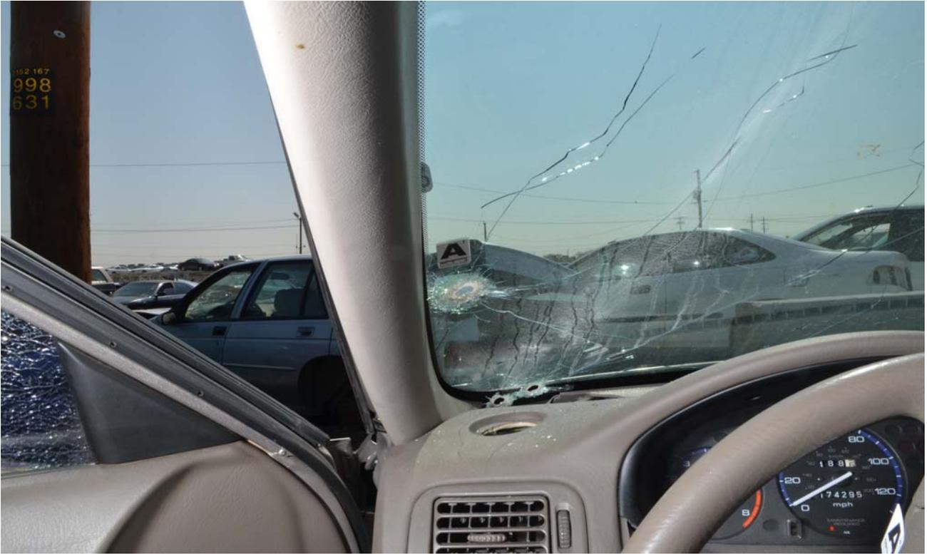
Two bullets struck the lower windshield and the dash. One bullet struck higher (A1) and struck the steering wheel housing (A2).
