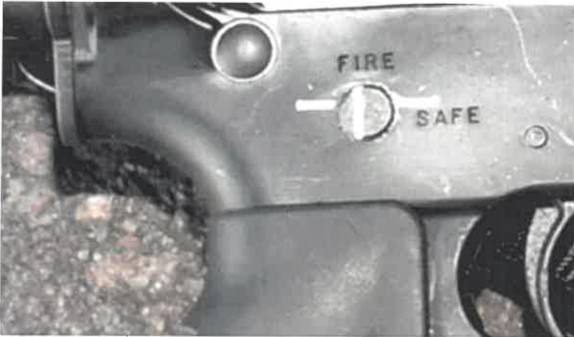
A closer view of the safety of the AR-15.
